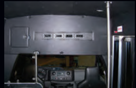
Black vinyl interior with optional drive modesty panel, stanchion and tinted plexiglass panel for added privacy
